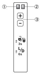
Function signal indicator (yellow), switching output
